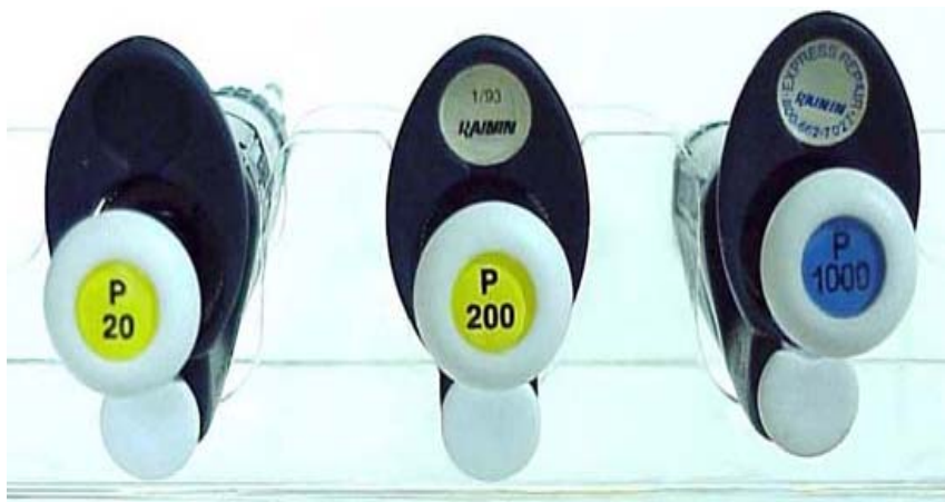
Figure 2 Top images of the P20, P200, and P1000: Micropipettors usually contain a label at the top of the device indicating the model. Modified image from University of Michigan-Dearborn.
