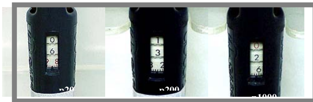
Figure 3 Volume Indicator Dials: The volume indicators are shown for a p20, p200, and p1000. Modified image from University of Michigan-Dearborn.
