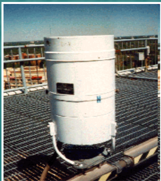
Typical HADS rain gauge
