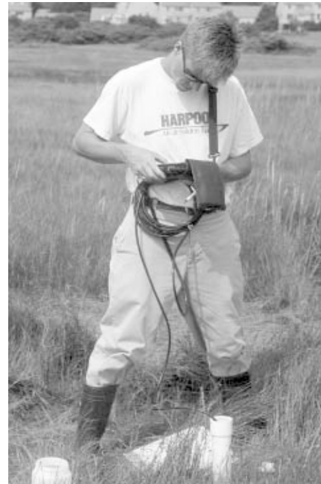
Measuring salinity with a digital multimeter.
