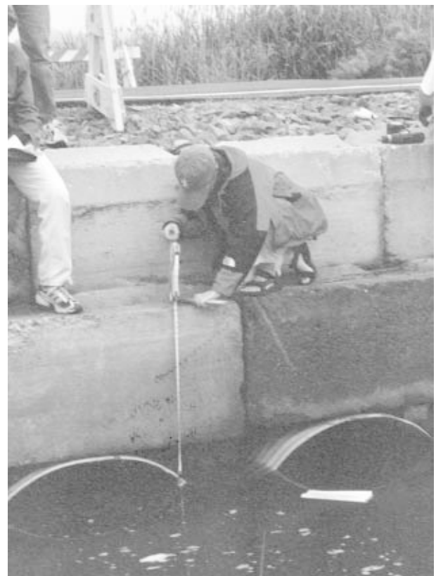
Measuring tidal height using the reference mark method.
